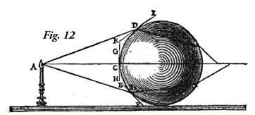
From this, you see that the rays can be brought together or spread apart, accordingly as they fall upon surfaces which are curved in various ways. And it is time that I begin to describe to you the structure of the eye, in order that you will be able to understand how rays which enter into it dispose themselves there to cause the sensation of sight.
